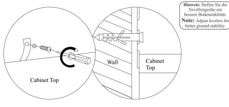
NOTE: Wall Fixings are not supplied with this product as different wall materials require different types of fixing devices (such as Rawl plugs on brick work) You must use fixing devices suitable for the type of wall you intend to mount this product to. Please ensure that the head of any screw used has a diameter greater than the diameter of the mounting hole on the product and that the fixing is safe and secure before use.
