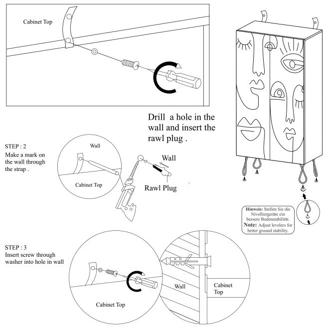
NOTE: Wall Fixings are not supplied with this product as different wall materials require different types of fixing devices (such as Rawl plugs on brick work) You must use fixing devices suitable for the type of wall you intend to mount this product to. Please ensure that the head of any screw used has a diameter greater than the diameter of the mounting hole on the product and that the fixing is safe and secure before use.
