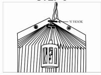
INSTALL THE HOOK "S" ON THE ELECTRICAL WIRE TO ADJUST AND FIX THE SOCKET IN THE CENTER OF THE SHADE
