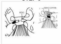
OPEN THE RING COVER TO PUT THE ELECTRICAL WIRE IN THE CENTER. CLOSE THE RING AFTER INSERTING THE WIRE .
