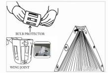
ADJUST THE BULB AND SOCKET ALONG WITH ELECTRICAL WIRE IN THE BULB PROTECTOR
