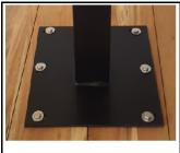
Secure the iron leg with Washer and bolts provided. Finger tighten all the bolts. Then fully tighten all boths with the help of wrench provided. Repeat these step for the second leg.
