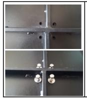
Fix the iron Base on the piller matching the holes.Secure the iron piller with Washer and bolts provided. Finger tighten all the bolts. Then fully tighten all boths with the help of wrench provided. Repeat these step for the second leg.
