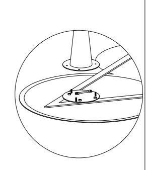
FIRSTLY,PLACE THE TOP UPSIDE DOWN.TAKE ONE LEG & MATCH THE HOLES AS SHOWN IN THE IMAGE.NOW SCREW THE LEG WITH THE GIVEN HARDWARE SET AS SHOWN IN CLOSE UP IMAGE. REPEAT THE SAME WITH OTHER 2 LEGS ALSO & THE WITH THE HELP OF AT LEAST 3 PEOPLE LIFT THE TABLE FROM THE TOP AND INSERT IT.
